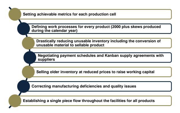
An especially critical function was to establish a lockdown production schedule to permit the plant to schedule raw material, tool changeovers, and manpower to match customer demand. This "pull" method of production significantly reduced waste in the system.
